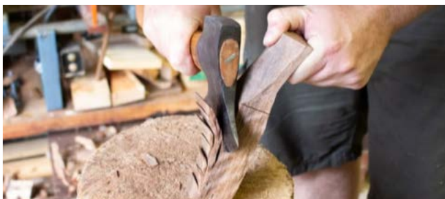
Figure 4: An axe can be used to rough out the shape of the spoon and remove excess bulk.
