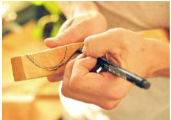
Figure 12: I had to re-draw the pattern on the block of wood several times as I corrected for errors and the way the blade was guided by the grain of the wood. The length of the face should be with the grain to minimise concerns and work with the wood.
