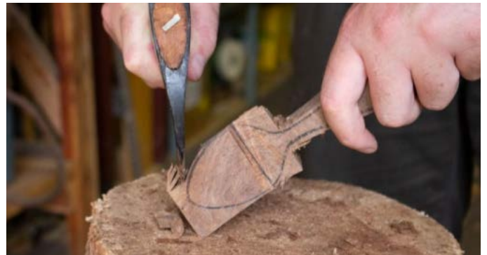
Figure 5: A sharp axe will allow for close cutting, reducing the amount of work needed with the knife.
