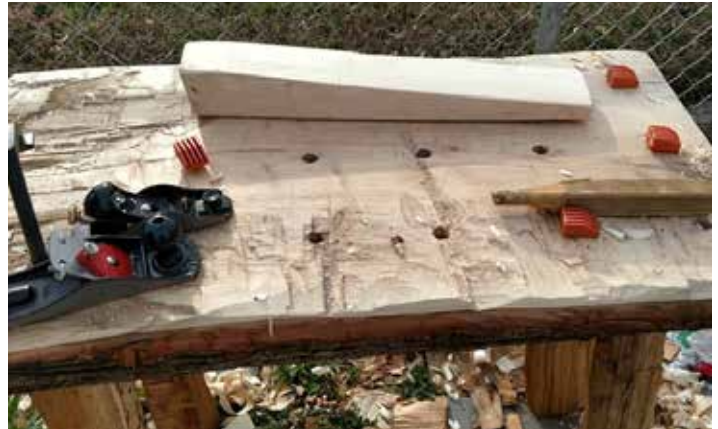
I bored holes for stops and holdfasts.
