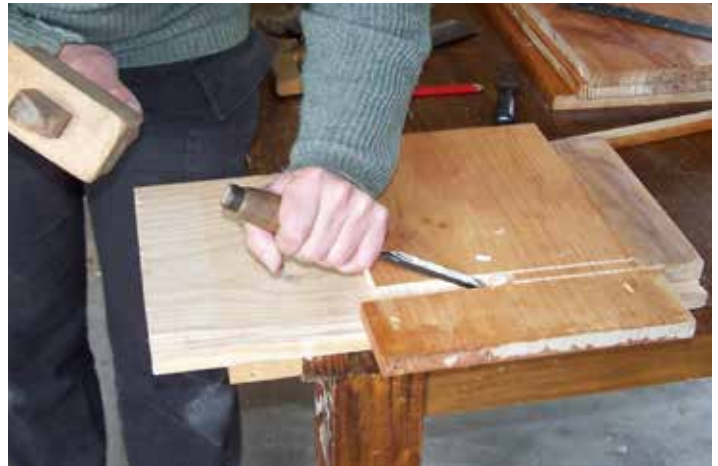
Smoothing out any high spots after removing most of the waste.
