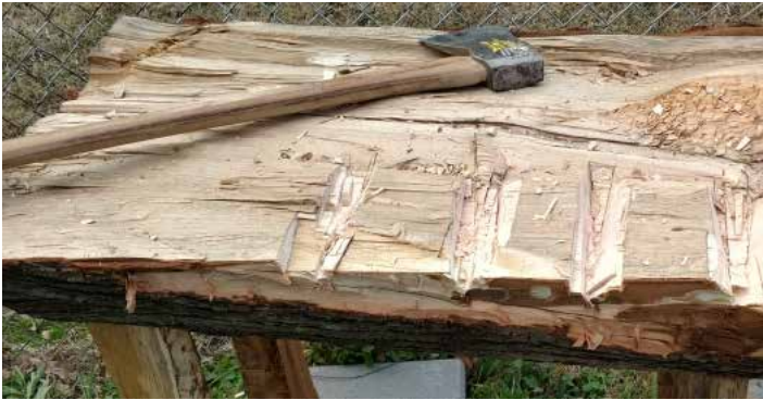
I used an axe to hew notches into the surface for rough material removal.
