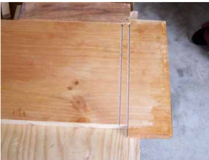
Braced against a bench stop, ready to chisel.
