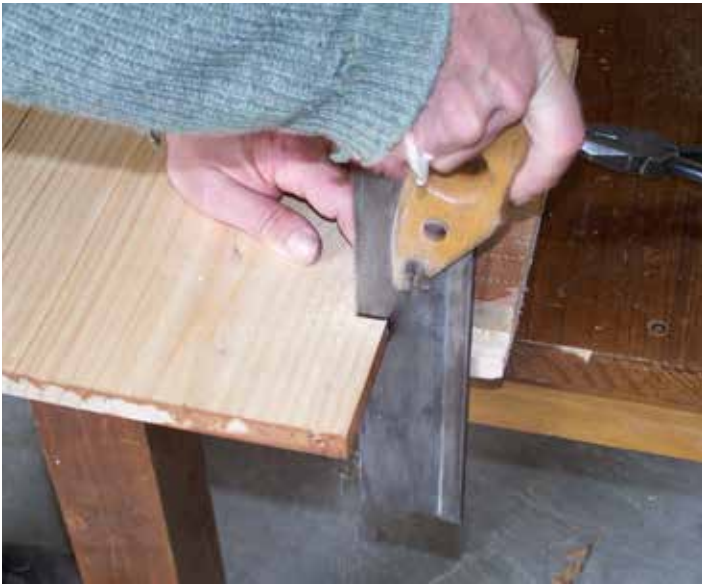
Cut, planed on the outside, ready to chisel the rebate/dado joint in the end board to take the base board.
