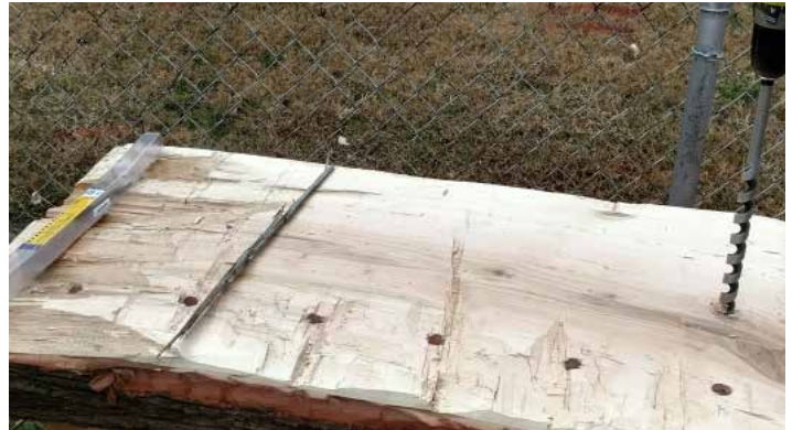
I bored holes for stops and holdfasts.
