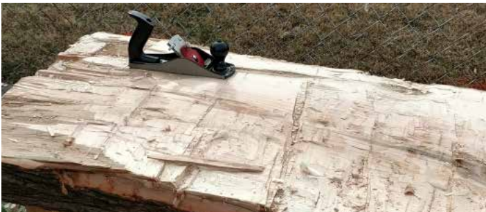
I have a lot to plane off. I don't have a scrub plane or a large jack plane, just this regular smoothing plane.
