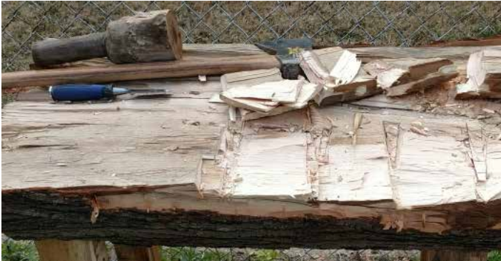
I used the axe and chisel to remove the joggles.
