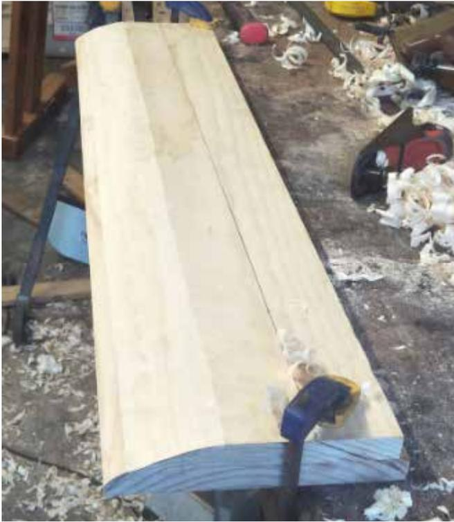
Planing a chamfer into the lids ends requires a jig to hold the work, I used a fixable timber slate and more clamps.
