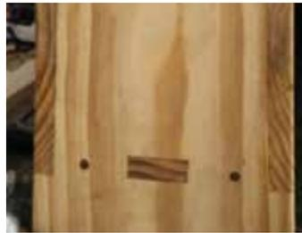
Note: In the photo to the left you can see how the grain is balanced by making the boards mirror each other to prevent warping. The tension with the grain pulls away equally.
