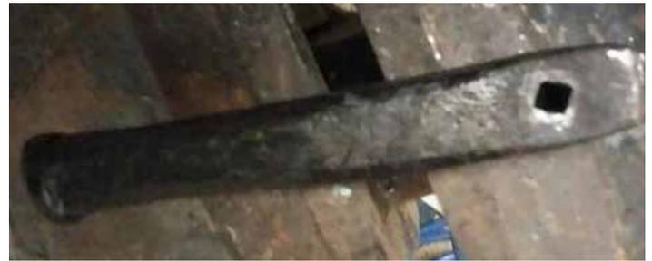
My copy in which I experimented with drifting a pyramid shaped hole.
