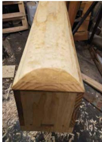
Once the top is dressed, turn the piece over and hollow out a trough till you reach the bottom of the top board. The goal is to have a constant thickness across the piece. I would recommend using a tool such as an adze or gauge. I personally used a spoon knife which was slow going and destroyed my hands.
