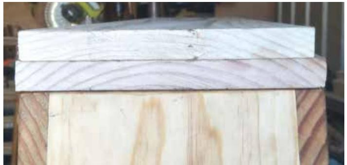
Once the boards are dry clamp on the work bench and plain the top face into a radius.
