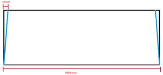
Repeating “Cut 2” we made to the End Walls we use the hand saw to angle the ends of side wall. This will allow the side walls to match flush with the end walls at which point we can glue the body together using soft wooden wedges to allow the clamps to sit square.
