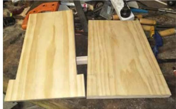
We will need to cut a rectangular mortise in the end walls in order to receive the floor plank.
