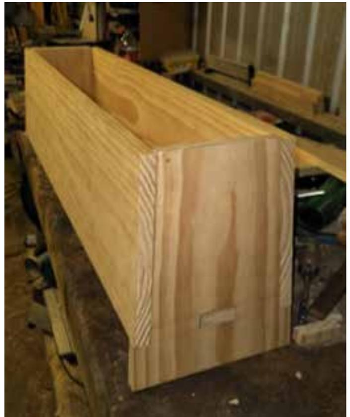
The edges of the floor board need to get trimmed with the block plane and carving knives into a trapezoid.
