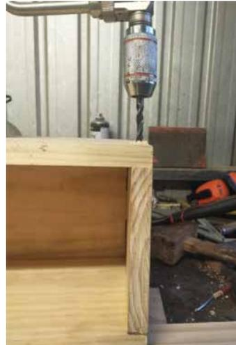
Once the hole is drilled apply glue then gently tape the dowel home with the mallet, then flush cut the dowel. Repeat, repeat, repeat... repeat, etc.
