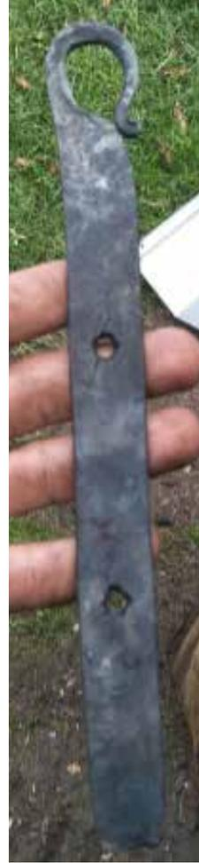
To forge the hinges, heat up your steel then hot cut 4 lengths of steel 200 mm long (I used a block splitter and hammer.) On all four pieces we round over one end and 2 holes punched in order to receive the clench nails.
