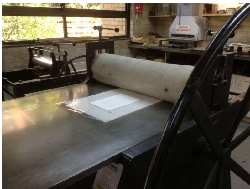
Inked matrix and paper on the bed of an intaglio press, about to be covered by the blankets
