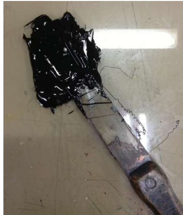
Working the ink to check for consistency and/or foreign objects
