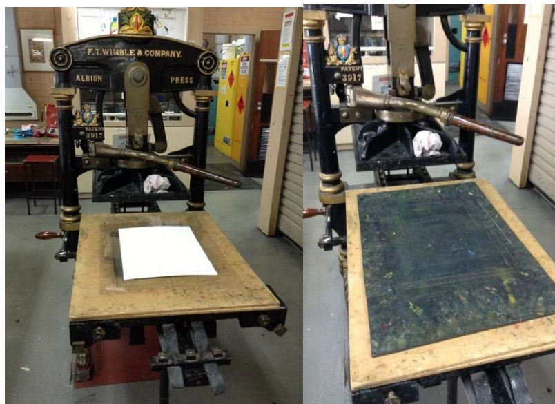
Above left: matrix and paper on the bed of the press, and right: rubber matting on top of both
