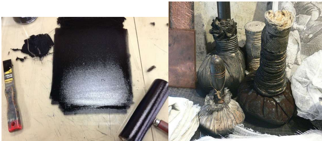
Above left: the modern printing brayer and right: inking balls from the Rembrandt museum
