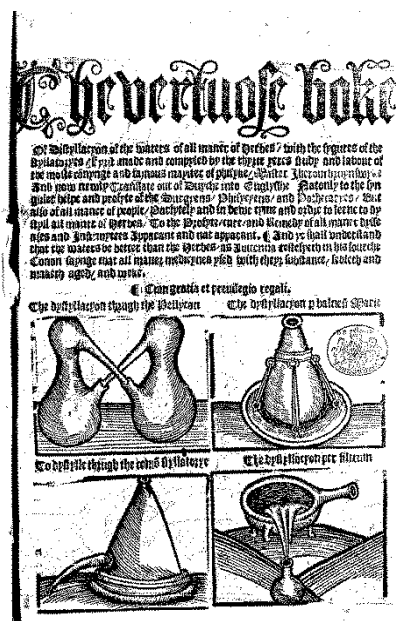
Figure 1: Title Page of the 1528 (3rd Edition) of The Virtuous Book of Distillation . Obtained from Early English Books Online database (June, 2014). Distillation equipment depicted on the cover are from the top left wood cuts of a Pelican , used to perform circulatory distillation; a flask in a balneum Marie , showing the weight and restraints to maintain submersion in the water bath; a common distillatory , placed over a large flask; and distillation per filtrum , an inexpensive approach to separate liquid from a herbal mash by meniscus flow down a linen cloth.
